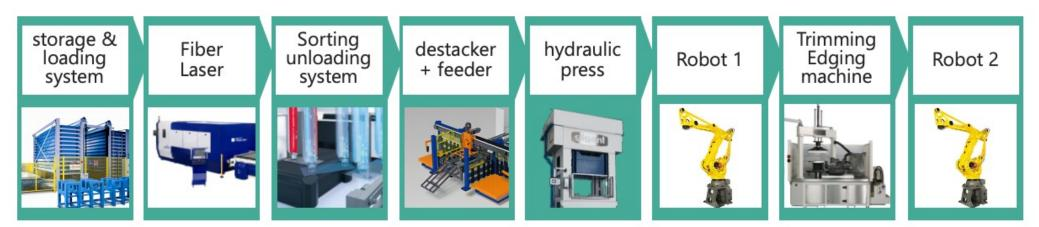
Laser-cutting and forming of aluminium products: a complex, automated manufacturing system where different technologies, different vendors and different control systems co-exist and cooperate.
